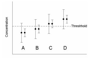
**Figure 1**. Schematic representation of how the uncertainty intervals (error bars) surrounding measurement results () affect the classification of batches of material against a regulatory threshold. A naive estimate of uncertainty, based only on
